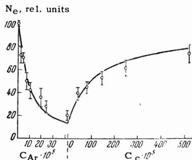
FIG. 3. Dependence of electron counting rate on the concentration of atoms of argon and, for a concentration of argon  $C_{Ar} = 4.2 \times 10^{-4}$ , on the concentration of carbon atoms.
