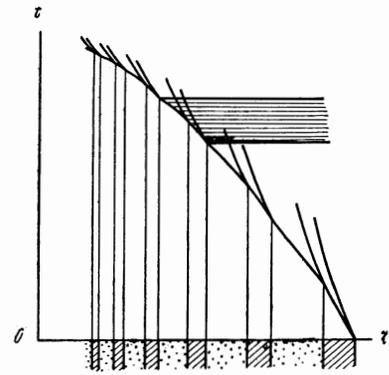
FIG. 3. Motion of a wave in a self-similar layered system.
