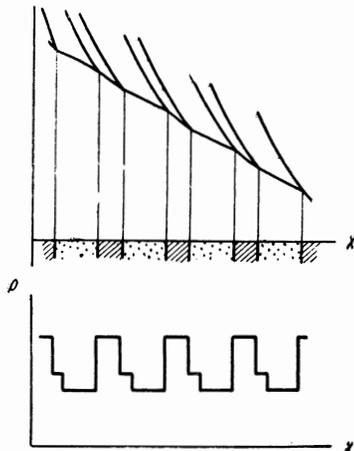
FIG. 2. Steady motion of a shock wave in a simple layered system;  $p$  = pressure on the front of the first wave.
