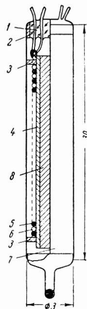
FIG. 1. Construction of the calorimeter used for sample  $\text{Gd}_{27}$ .
