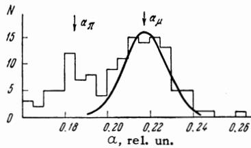
FIG. 1. Distribution of primary tracks in pion and muon stars as a function of the parameter  $\alpha$ , for experiment 4. The smooth curve is the resolution function for muon stars.
