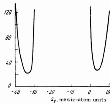
FIG. 7. Plot of  $\chi^2$  for the  $l$  distributions of experiments 1–3, as a function of the scattering length  $a_g$ , computed by the Monte-Carlo method.
