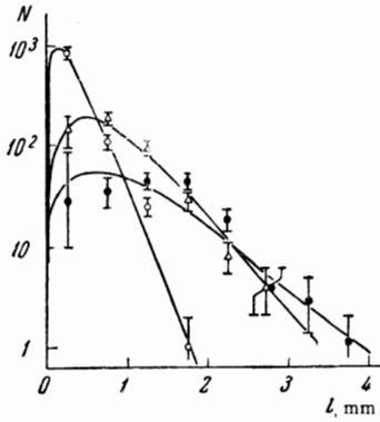
FIG. 5. Experimental distributions of events in range for  $p\mu$  atoms:  $\circ$  – in experiment 1,  $\Delta$  – in experiment 2,  $\bullet$  – in experiment 3. The smooth curves are calculated by the Monte-Carlo method with the parameters listed in Table III.
