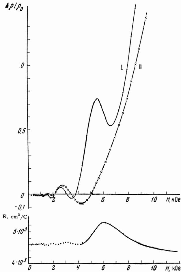
FIG. 2. Experimental curves of the dependences of the transverse and longitudinal magnetoresistance and of the Hall coefficient on the magnetic field intensity for sample No. 2. In  $H < 4$  kOe, the electron density  $n = 1.35 \times 10^{15} \text{ cm}^{-3}$ , and the mobility  $u = 1.1 \times 10^5 \text{ cm}^2 \cdot \text{V}^{-1} \cdot \text{sec}^{-1}$ ; the temperature was  $T = 1.4^\circ\text{K}$ .
