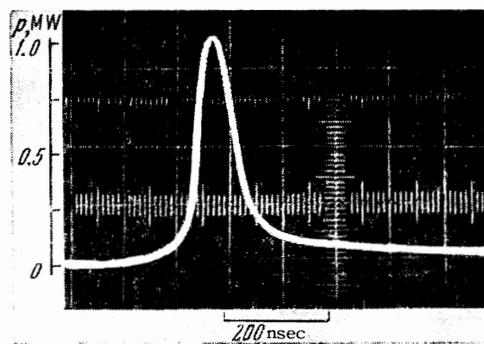
FIG. 2. An oscillogram of a single laser pulse obtained with a solution of free base phthalocyanine in quinoline.
