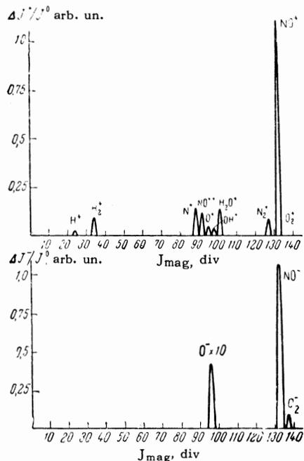
FIG. 2. Mass spectrum of slow positive and negative ions formed in NO.
