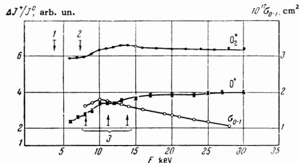
FIG. 7. The process  $H^0 \rightarrow H^-$  in O<sub>2</sub>: 1 —  $H^0 + O_2 \rightarrow H^- + O_2^+$ ; 2 —  $H^0 + O_2 \rightarrow H^- + O_2^+ [{}^2\Pi_u]$ ; 3 —  $H^0 + O_2 \rightarrow H^- + (O_2^+)^* \rightarrow H^- + O^+ + O^*$  (the O atom is found in the ground state and excited states).
