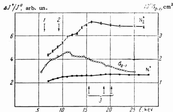
FIG. 6. The process  $H^0 \rightarrow H^-$  in N<sub>2</sub>: 1 —  $H^0 + N_2 \rightarrow H^- + N_2^+$ ; 2 —  $H^0 + N_2 \rightarrow H^- + N_2^+ [{}^2\Sigma_u^+]$ ; 3 —  $H^0 + N_2 \rightarrow H^- + (N_2^+)^* \rightarrow H^- + N^* + N^+$  (the N atom is found both in the ground state and in excited states).
