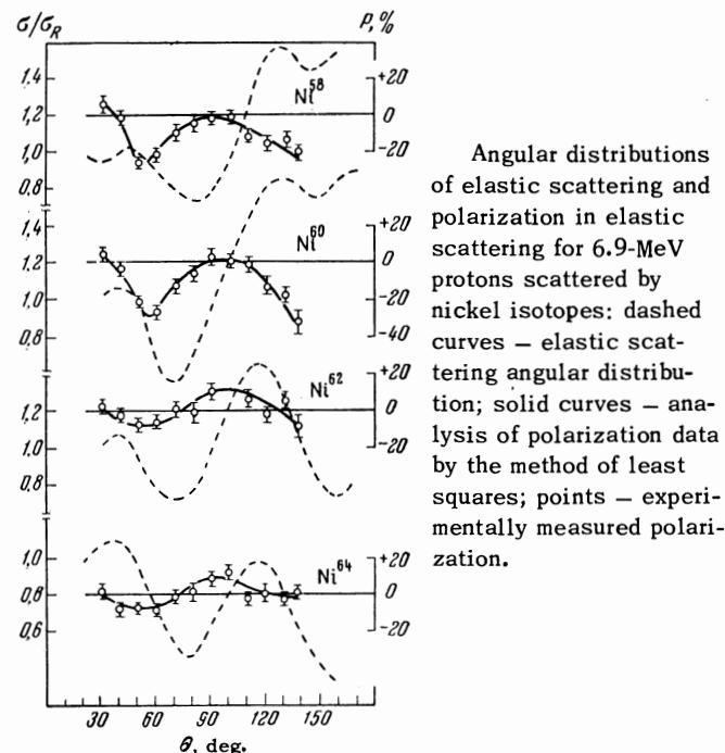
For observation of the difference in the polarization arising in scattering of protons by different nuclei, it was sufficient to measure the product  $P_1 P_2$ , where  $P_1$  and  $P_2$  are respectively the desired polarization and the polarization of the analyzer. Using Rosen's data, [8] we evaluated  $P_2$  and computed  $P_1(\theta)$ .
