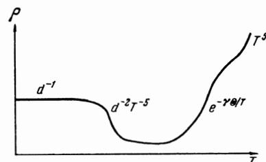
FIG. 1. Resistance of thin sample.
