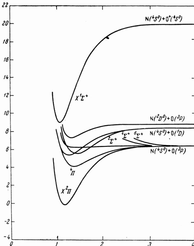
Potential curves of  $V(R)$  ( $V$  in eV,  $R$  in Å) of the systems  $N + O$  and  $NO^+$ .
