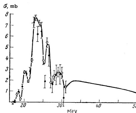
FIG. 1. Differential cross section for the reaction  $C^{13}(\gamma, p)B^{12}$ . The hollow circles indicate average values of three independent series of measurements; the solid circles refer to a separate series of measurements obtained at intermediate energy values.
