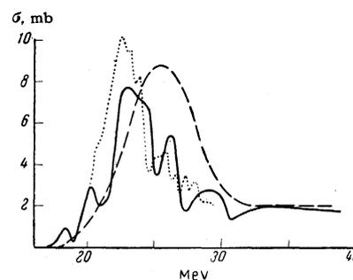
FIG. 2. Comparison of our experimental differential cross section curve for the reaction  $C^{13}(\gamma, p)B^{12}$  (solid curve) with the curve obtained by Cook<sup>[1]</sup> (dashed curve), and with the curve obtained by Dodge and Barber<sup>[2]</sup> (dotted curve) for the cross section of the  $C^{12}(\gamma, p)B^{11}$  reaction.
