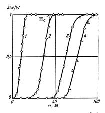
FIG. 1. Superconducting transition curves of zirconium: 1)  $T = 0.145^{\circ}K$ ; 2)  $T = 0.47^{\circ}K$ ; 3)  $T = 0.242^{\circ}K$ ; 4)  $T = 0.35^{\circ}K$ ; 0-without pressure;  $\triangle - p = 16$  300 atm.
