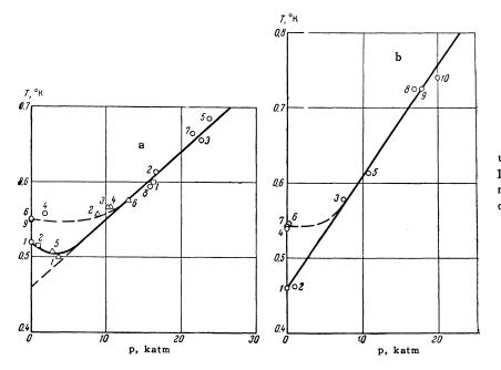
FIG. 3. Dependence of  $T_c$  on pressure: a) unannealed zirconium samples (O-sample No. 1,  $\triangle$ -sample No. 2, D-sample No. 3); b) annealed zinc samples. Numbers at the points denote the sequence of compression cycles.
