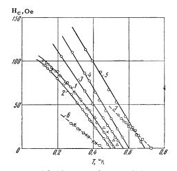
FIG. 2. Critical field curves of unannealed (continuous curves) and annealed (dashed curves) zirconium samples. 1) Without pressure: O-initial sample,  $\times$ -after fifth and  $\triangle$ -after eighth compression cycle (cf. Fig. 3a, sample No. 1); 2) p = 3700 atm (sample No. 2); 3) p = 8800 atm (sample No. 2); 4) p = 16 300 atm (sample No. 3); 5) p = 23 600 atm (sample No. 1); 6) without pressure: D-initial sample,  $\times$ -after second compression cycle (Fig. 3b); 7) p = 18 000 atm.
