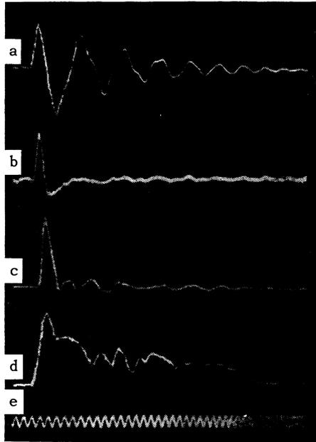
FIG. 2. Oscillograms: (a) electric field  $E_\theta$ , (b) plasma current, (c) hard x-ray component, (d) emission of the  $H_\alpha$  line recorded by the photomultiplier 12. The calibration oscillogram d shows a sine wave at a frequency of 12 Mc/sec. All oscillograms are taken at a plasma density  $n_{\text{int}} \approx 1 \times 10^{12} \text{ cm}^{-3}$  and have the same time scale.
