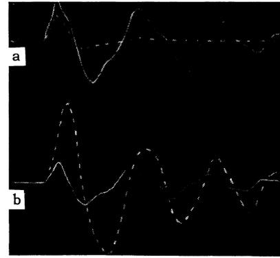
FIG. 3. Comparison of the oscillograms for the current (dotted) and electric field (solid): (a) for a toroidal chamber containing plasma, (b) for a copper torus.
