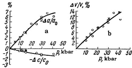
FIG. 1. a) Dependence of the linear compressibility of tellurium on pressure. Circles denote x-ray diffraction data, crosses give Bridgman's data<sup>[7]</sup>; b) dependence of the volume compressibility of tellurium on pressure. Circles denote x-ray diffraction data, crosses give Bridgman's data.<sup>[7]</sup>
