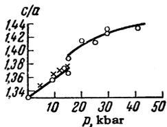
FIG. 2. Dependence of  $c/a$  on pressure. Circles denote x-ray diffraction data (for the A7 phase at  $p = 15$  kbar  $c/2a$  was used), and crosses denote the values of  $c/a$  calculated from Bridgman's data.<sup>[7]</sup>
