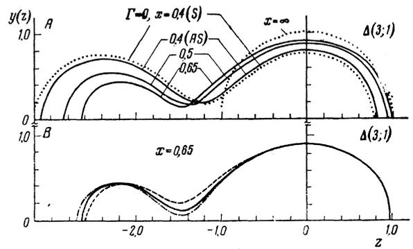
FIG. 4. Asymmetric absolute equilibrium shapes (saddles) of type (3; 1). Solid lines represent  $\Gamma = 0$ , dotted lines represent  $\Gamma = + 0.1$ , the dash-dotted lines represent  $\Gamma = - 0.1$ . In case A the dots indicate the contour of symmetric AE shape for  $x = 0.4$  ( $\Gamma = 0$ ), and also the sphere of unit radius.
