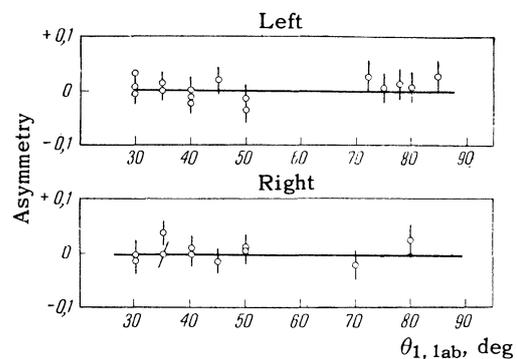
crystals [0.8 and 1.4 mm CsI(Tl)], after amplification and clipping, were fed to a gating circuit and then to a multichannel pulse-height analyzer. To take into account any spurious asymmetry, the measurements were carried out to the left and to the right of the primary deuteron beam.
