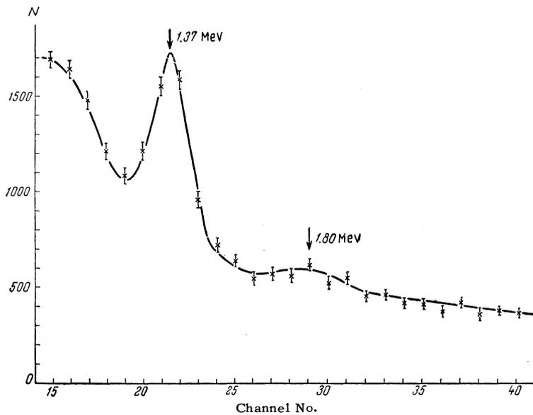
FIG. 3. Apparatus spectrum of  $\gamma$  quanta generated in inelastic scattering of 14-MeV neutrons by magnesium.
