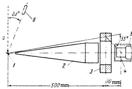
FIG. 2. Geometry of the experiment: 1 – neutron source; 2 – lead shield; 3 – scatterer; 4 – scintillator of  $\gamma$  spectrometer; 5 – photomultiplier; 6 – proportional counter for  $\alpha$  particles.
