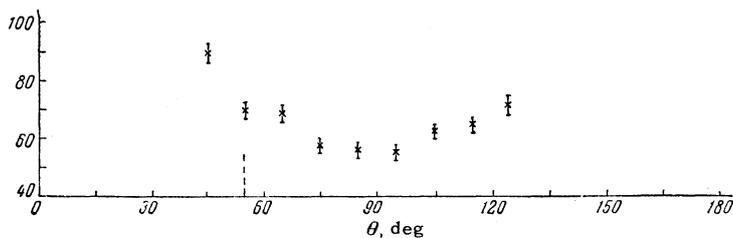
FIG. 5. Angular distribution of 1.37-MeV  $\gamma$  quanta generated by inelastic scattering of neutrons by magnesium.
