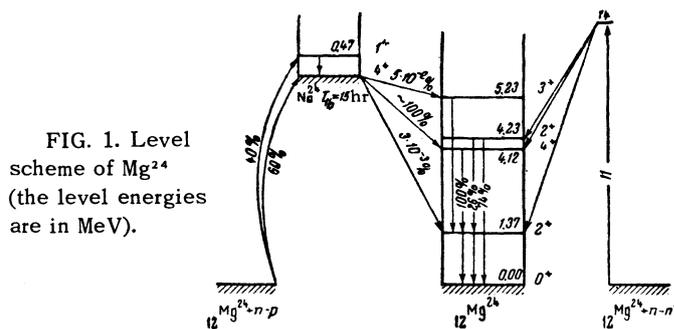
FIG. 1. Level scheme of Mg<sup>24</sup> (the level energies are in MeV).
