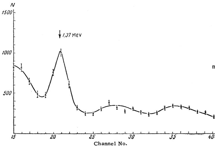
FIG. 4. Apparatus spectrum of  $\gamma$  quanta from a sample of magnesium activated with 14-MeV neutrons.
