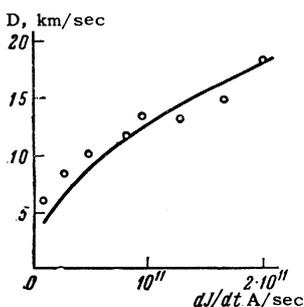
FIG. 4. Dependence of the velocity of broadening of the spark channel in air (1 atm) on the rate of current rise;  $l = 0.2$  mm.
