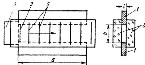
FIG. 1. Construction of the gap: 1) metal electrodes; 2) transparent side jaws; 3) wire for location of the breakdown spot; 4) restricting plate; 5) scale marks. Typical dimensions:  $a = 20$  mm;  $b = 5$  mm;  $l = 0.2$  mm.
