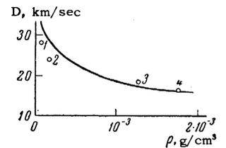
The maximum velocity in a gas at 1 atm for a gap of 0.2 mm width at  $dJ/dt = 2 \times 10^{11}$  A/sec was 18 km/sec for air and 28 km/sec for hydrogen.
