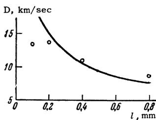
FIG. 3. Dependence of the velocity of broadening of the spark channel in air (1 atm) on the gap width;  $dJ/dt = 1.6 \times 10^{11}$  A/sec.
