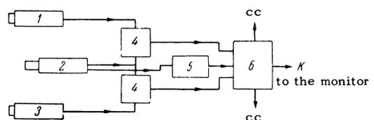
FIG. 2. Block circuit of the electronics: 1, 3 – crystal neutron detectors, 2 – scintillation gas counter, 4 – two-channel fast-coincidence circuit, 5 – differential discriminator, 6 – slow-coincidence circuit, cc – counting circuits.
