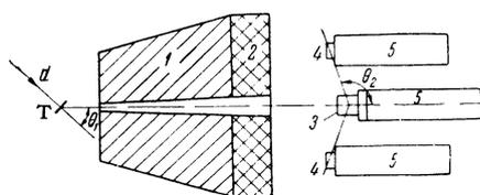
FIG. 1. A schematic diagram of the setup for investigating the polarization: T – target, 1 – paraffin cone, 2 – lead shield, 3 – scintillation gas counter, 4 – crystal neutron detectors, 5 – photomultipliers.
