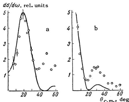
FIG. 2. Angular distributions of protons from the  $\text{Mo}^{94}(\text{d}, \text{p})\text{Mo}^{95}$  reaction: a – for transitions to the ground and excited (0.2-MeV) state of  $\text{Mo}^{95}$  ( $l_n = 2$ ), b – for transitions to a number of states with energies 0.77-1.0 MeV ( $l_n = 0$ ). In both cases  $r_0 = 6.2$  F.
