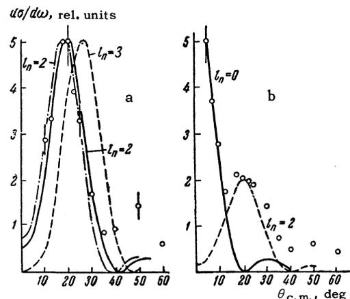
FIG. 1. Angular distributions of protons for the  $\text{Mo}^{92}(\text{d}, \text{p})\text{Mo}^{93}$  reaction: a – for the transition to the ground state of  $\text{Mo}^{93}$ , b – for the transition to the first excited (0.91-MeV) state. The curves were calculated by the simple stripping theory; the values of  $l_n$  are indicated on the curves,  $r_0 = 6.0 \text{ F}$ .
