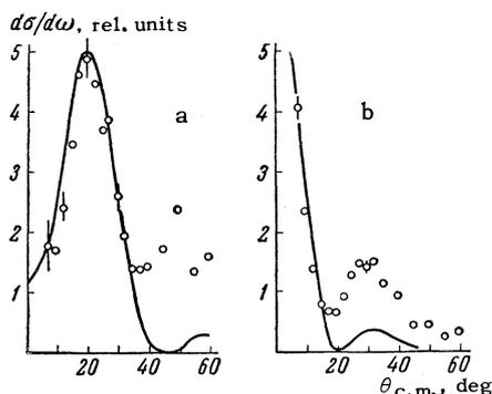
FIG. 4. Angular distribution of protons from the  $\text{Mo}^{96}(\text{d}, \text{p})\text{Mo}^{97}$  reaction: a— for transitions to the ground state ( $l_n = 2$ ), b— for transitions to the excited (0.66-MeV) state ( $l_n = 0$ ); in both cases  $r_0 = 5.8 F$ .
