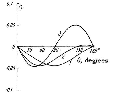
FIG. 1. Function  $P_{l'}(\theta)$  for tungsten. 1 - elastic polarization, 2 - polarization in inelastic scattering with excitation of the level  $l=2$ , 3 - the same with excitation of the level  $l=4$ .
