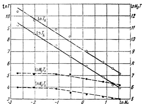
FIG. 4. Dependence of  $T_{\parallel}$ ,  $T_{\perp}$ ,  $N_S T_{\parallel}$ ,  $N_S T_{\perp}$  on the concentration of paramagnetic atoms (for VOSO<sub>4</sub>).
