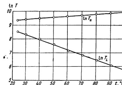
FIG. 2. The temperature dependence of  $T_{\parallel}$  and  $T_{\perp}$  for a paramagnetic atom concentration of  $N_S = 0.1$  mole/liter ( $\text{VOCl}_2$ ). The points denote experimental values, the solid lines calculated values.
