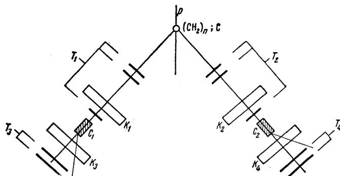
FIG. 1. Schematic diagram of the experiment for measurement of  $C_{kp}$ :  $C_1$  and  $C_2$  - analyzing target;  $K_1, K_2, K_3, K_4$  - gas discharge chambers;  $T_1, T_2, T_3, T_4$  - scintillation counter telescopes.
