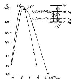
FIG. 2. Coincidence curves (one of five series) for Gd<sup>149</sup> and Co<sup>60</sup> sources, taken with a pair of stilbene crystals.
