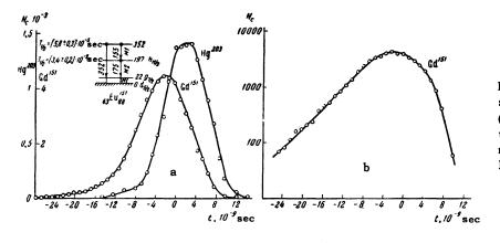
FIG. 4. Coincidence curves for  $Gd^{151}$  and  $Hg^{203}$  sources, taken with the energy intervals shown in Fig. 3, in ordinary (a) and logarithmic (b) scale. The source was deposited on a  $10\mu$  thick aluminum backing, which freely transmits the K conversion electrons of the 175-keV line.
