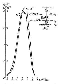
FIG. 1. Coincidence curves (one of six series) for sources of Gd<sup>147</sup> (decay scheme shown in insert) and Na<sup>22</sup>, taken with a pair of NaI (Tl) crystals with the same energy intervals.
