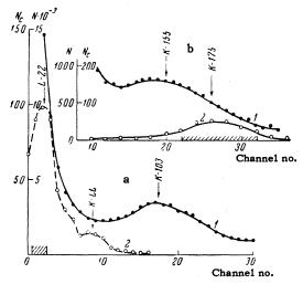
FIG. 3. Spectrum of conversion electrons from a Gd<sup>151</sup> + Gd<sup>153</sup> source. a) region of the 21.7-keV transition: 1) singles spectrum, 2) spectrum of electrons coincident with the K line of 175 keV; b) region of the 175-keV transition: 1) singles spectrum, 2) spectrum of electrons coincident with the 21.7 keV L conversion line for a delay of 20 nsec. The crosshatching on the abscissa shows the position of the "windows" of the pulse analyzers in the time measurements.
