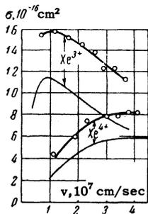
Cross section for single-electron charge exchange of Xe<sup>3+</sup> and Xe<sup>4+</sup> in Ne as functions of velocity  $v$ . Heavy curves—experimental; thin curves—calculated.
