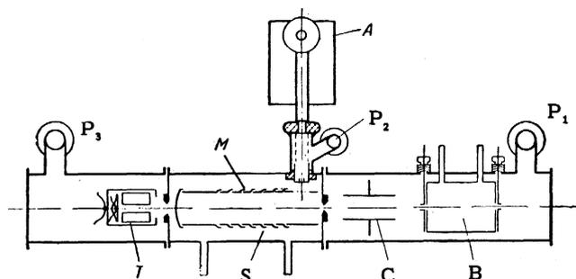
FIG. 1. Experimental setup: B is the chamber where an atomic beam is formed by charge exchange; C is the capacitor where charged particles are removed from the atomic beam; S is the scattering chamber; M is the measuring capacitor; T is the receiver of fast particles; A is the analyzer of slow ions;  $P_1$ ,  $P_2$ ,  $P_3$ , are pumps.
