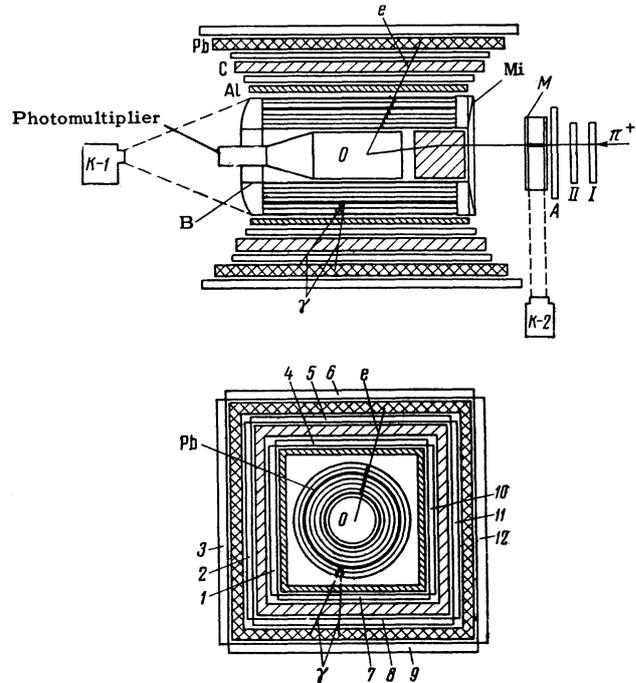
Diagram of equipment used to register  $\mu \rightarrow e + \gamma$  decays. B—6-layer cylindrical spark chamber, M—single-layer flat spark chamber, K-1, K-2—motion picture cameras; Mi—mirrors to produce a stereoscopic picture of the event in the chamber. O, I, II, A, 1–12—scintillation counters. The apparatus was shielded with lead and paraffin with boron on all sides
