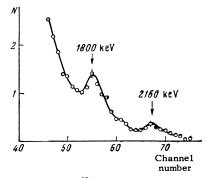
FIG. 12.  $\gamma$  spectrum of V<sup>47</sup>, measured with a lead filter 25 mm thick.
