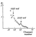
FIG. 10.  $\gamma$  spectrum of Mn<sup>51</sup>, measured with a lead filter 25 mm thick.
