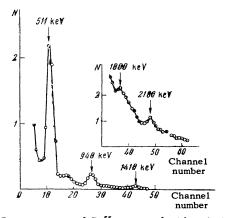
FIG. 5.  $\gamma$  spectrum of Co<sup>55</sup> measured with scintillation  $\gamma$  spectrometer. The hard portion of the  $\gamma$  spectrum, measured with a 25-mm lead filter, is shown in the upper right corner.
