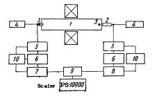
FIG. 1. Block diagram of setup for measuring  $\beta\gamma$  coincidences: 1-magnetic spectrometer, 2-photomultiplier, 3-end-window counter, 4-high-voltage source, 5-cathode follower, 6-amplifier, 7-delay block, 8-differential analyzer, 9-coincidence circuit, 10-rectifier (200 V), S-radio-active source.
