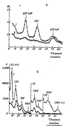
FIG. 15.  $\gamma$  spectrum of Se<sup>83</sup> + Br<sup>82</sup>; a – soft part of the spectrum, b – hard part. Lower curves correspond to the  $\gamma$  spectra measured after several hours.
