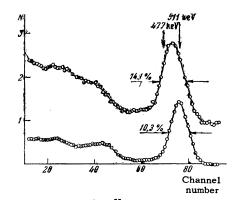
FIG. 6.  $\gamma$  spectrum of Co<sup>55</sup> (upper curve) and  $\gamma$  spectrum of annihilation radiation of Cu<sup>54</sup> (lower curve), measured with conical lead collimator.
