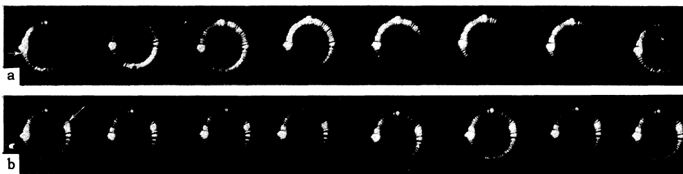
FIG. 3. Photographs of a discharge with p = 2 \times 10^{-2} mm Hg. The traveling wave moves in the counterclockwise direction: (a) discharge without magnetic mirror (the arrow indicates the beginning of the delay line) b) discharge with a magnetic mirror field H_{\text{mir}} = 125 Oe (the arrow indicates the position of the magnetic mirror).
