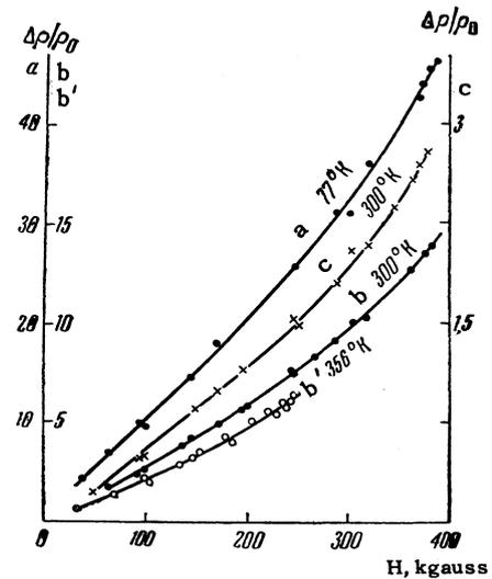
FIG. 3. The dependence of magnetoresistance on the magnetic field intensity for two samples of InAs: G1 (curves a, b, and b') and M-13 (curve c).
