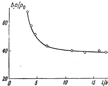
FIG. 2. The dependence of magnetoresistance on the parameter  $l/b$  for sample G1;  $l$  is the length of the sample and  $b$  is its width.  $H = 350$  kgauss,  $T = 77^\circ\text{K}$ .
