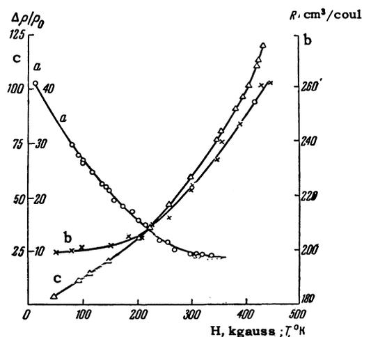
FIG. 4. Sample G1: a) the dependence of magnetoresistance on temperature ( $H = 252$  kgauss); b) the dependence of the Hall coefficient on the magnetic field intensity ( $T = 20^\circ\text{K}$ ); c) the dependence of magnetoresistance on the magnetic field intensity ( $T = 20^\circ\text{K}$ ).
