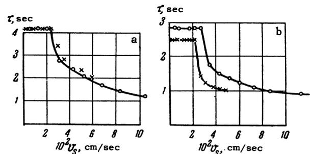
FIG. 3. Dependence of  $\tau$  upon the velocity  $v_s$ :  $\times$  - counterflow case,  $\circ$  - case of flow only of superfluid component. a -  $T = 1.44^\circ$  K; for both cases  $W_2 = 5.5 \times 10^{-2}$  w/cm<sup>2</sup>, b -  $T = 1.32^\circ$  K;  $W_2 = 6.5 \times 10^{-2}$  w/cm<sup>2</sup> for counterflow and  $W_2 = 5.5 \times 10^{-2}$  w/cm<sup>2</sup> for motion of the superfluid component alone.
