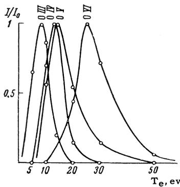
FIG. 4. Calculated dependence of the relative intensities of the OIII, OIV, OV, and OVI lines on the electron temperature of the plasma (wavelength of the OVI line is equal to 1036 Å).
