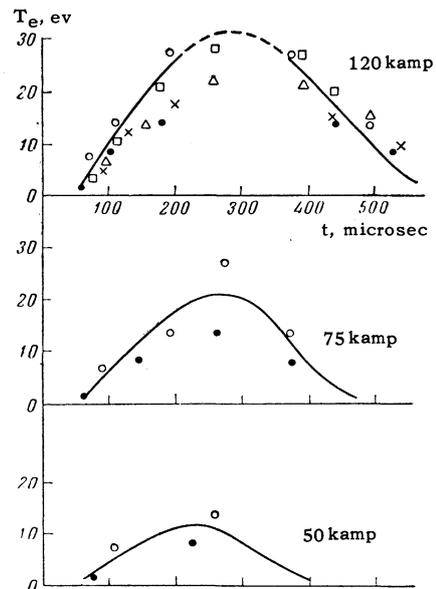
FIG. 5. Time dependence of the electron temperature for different values of the maximum discharge current determined from different lines:  $\circ$  – OV,  $\bullet$  – OIII,  $\square$  – FV,  $\triangle$  – FIV,  $\times$  – FIII.
