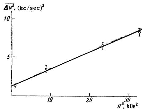
FIG. 2. Dependence of the second moment of the  $\text{Sn}^{119}$  absorption line on the square of the external magnetic field.
