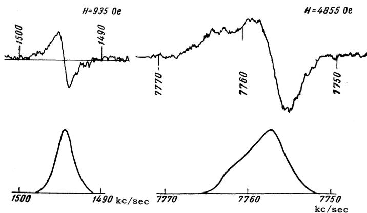
FIG. 1. Upper, derivative traces of  $\text{Sn}^{119}$  absorption lines; lower, integrated line shapes.
