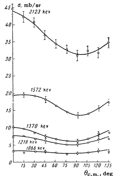
**FIG. 5.** Angular distributions of neutrons from  $\text{F}^{19}(t, n)$  for different triton energies.
