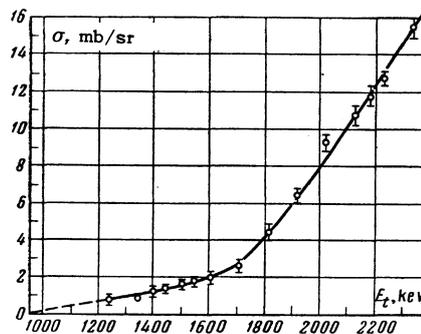
FIG. 3. Differential cross section for neutron yield from  $Al^{27}(t, n)$ .
