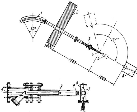
FIG. 1. Diagram of apparatus. 1 - magnetic analyzer, 2 - paraffin-borax shield, 3 - closure, 4 - target, 5 - 30-cm copper cone, 6 - neutron counter, 7 - target holder, 8 - T tube 0.2 mm thick, 9 - collimator diaphragms.
