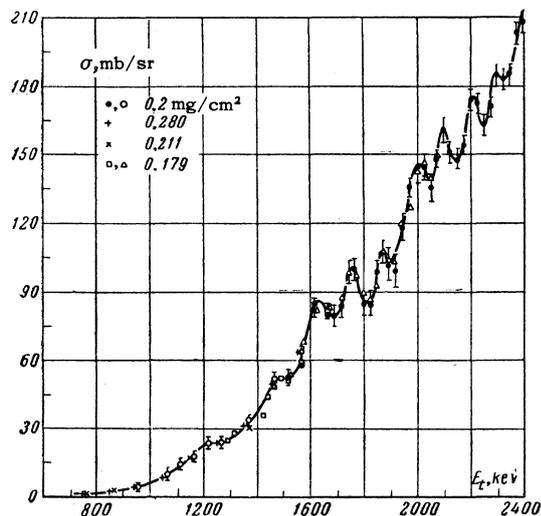
FIG. 2. Differential cross sections for neutron yield at  $0^\circ$  angle from triton reactions with aluminum fluoride targets of different thicknesses.  $E_t$  is triton energy.
