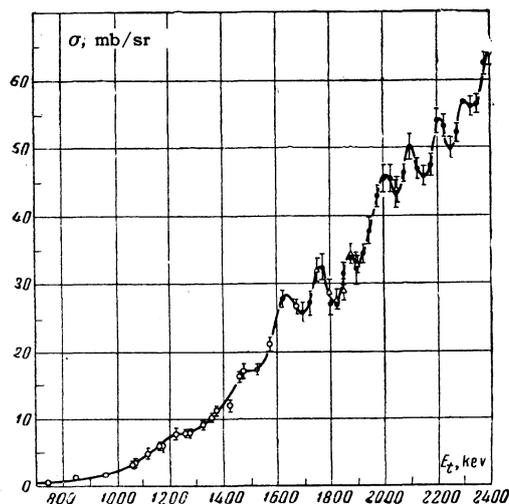
FIG. 4. Differential cross section for neutron yield at  $0^\circ$  angle from  $F^{19}(t, n)$  vs triton energy.
