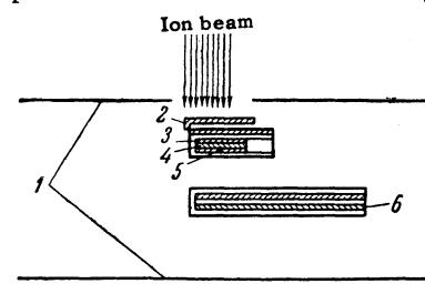
Experimental arrangement: 1—dee; 2—target; 3—copper; 4—graphite; 5—iron; 6—detector for measurement of the neutron angular distribution.
