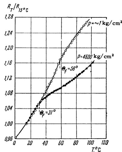
FIG. 2. The temperature dependence of the electrical resistivity of CrTe at atmospheric pressure and at  $p = 4,600 \text{ kg/cm}^2$ .
