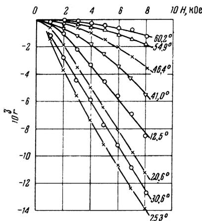
FIG. 3. Isotherms of the electrical resistivity change of CrTe with magnetic field at a pressure of  $4,600 \text{ kg/cm}^2$ .
