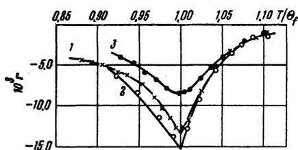
FIG. 6. Temperature dependence of the transverse galvanomagnetic effect at  $H = 8000$  oe: curve 1—CrTe at atmospheric pressure, curve 2—CrTe at  $p = 4,600 \text{ kg/cm}^2$ , curve 3—CrTe<sub>0.93</sub>Se<sub>0.07</sub> at atmospheric pressure.
