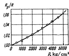
FIG. 1. The influence of pressure on the electrical resistivity of CrTe at room temperature; x - pressure increasing, o - pressure decreasing.
