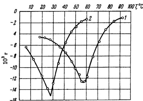
FIG. 4. Temperature dependence of the galvanomagnetic effect: curve 1 – at atmospheric pressure, curve 2 – at a pressure of  $4,600 \text{ kg/cm}^2$ .
