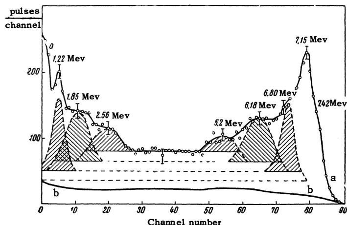
FIG. 1. a - Coincidence spectrum of captured  $\gamma$  radiation of  $Nd^{144}$ , occurring when the capture is in the energy range 1-8 Mev (rms errors); b - spectrum of random coincidences under the same conditions.
