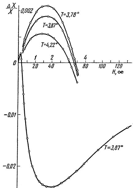
magnetic field which was parallel to the axis of the coil and the specimen. Along the ordinate axis is plotted the relative change of the reactive component of the impedance relative to the total magnitude, the latter being determined from the change in the oscillator frequency when the sample has passed into the superconducting state. In the top portion of the diagram are plotted the first parts of the curves at various temperatures on a larger scale.
