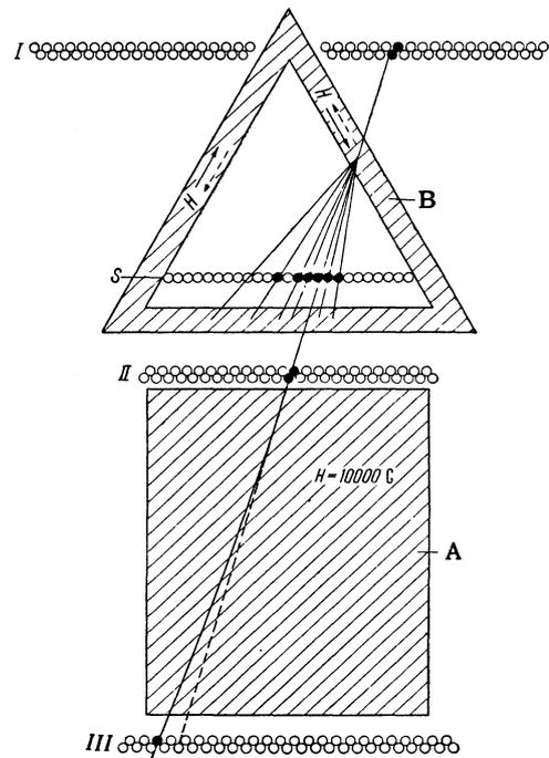
I, II, and III are rows of hodoscopic counters for the determination of the trajectory of the  $\mu$  meson. S is a row of counters for the registration of the showers. A is the iron yoke of a permanent magnet for the determination of the sign of the  $\mu$  mesons from the deflection in a magnetic field. B is the iron core of an electromagnet with a triangular cross-section, in which the  $\mu$  mesons produced showers, including some on electrons polarized by the magnetic field.
