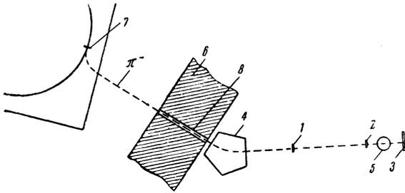
FIG. 1. Experimental setup (schematic): 1, 2, 3 – scintillation counters, 4 – deflecting magnet, 5 – hydrogen scatterer, 6 – yoke of the synchrocyclotron magnet, 7 – beryllium target inside the synchrocyclotron chamber, 8 – pion collimator.
