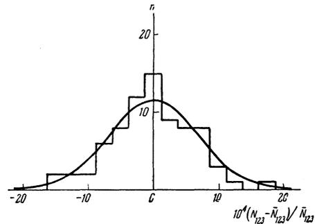
FIG. 2. The spread of the deviations of the normalized coincidence count  $N_{123}$  (with hydrogen) from the mean value;  $n$  is the number of measurements having a given deviation; the solid curve is the distribution function calculated on the assumption that the deviations are due only to statistical fluctuations.
