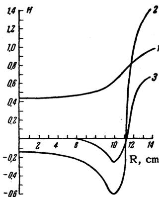
FIG. 1. Discharge in hydrogen,  $p = 0.05$  mm Hg. Curve 1 - magnetic field in the absence of a discharge, 2 - magnetic field during the second half cycle of current, 3 - during the third half cycle.
