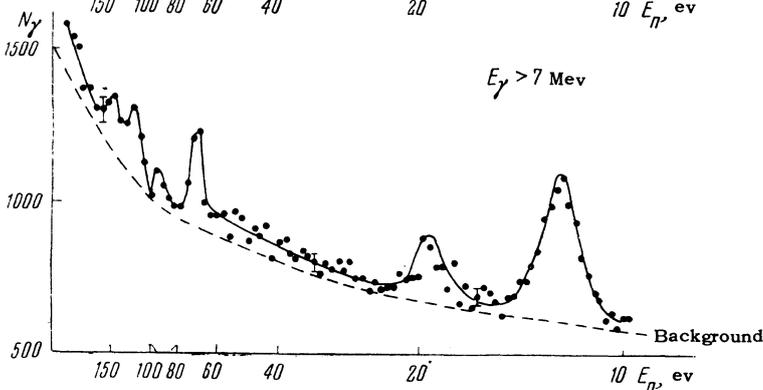
FIG. 3. Intensity of resonances of  $\text{Pt}^{195}$  at different energies of registered capture  $\gamma$  rays,  $N_\gamma$  – number of pulses.
