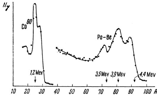
FIG. 2. Calibration curves for NaI(Tl) crystals. A – pulse amplitude in relative units,  $N_\gamma$  – number of pulses in relative units.
