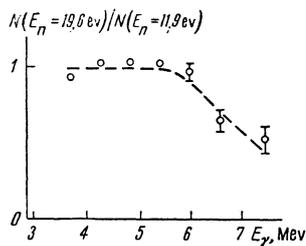
FIG. 5. Comparison of intensity of  $\gamma$ -ray spectra for the 19.6- and 11.9-ev resonances.
