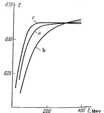
**FIG. 2.** Variation of efficiency  $\epsilon$  of registration of  $\gamma$  quanta with their energy  $E$ .
