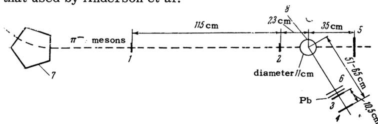
FIG. 1. Geometry of the charge-exchange scattering experiment: 1, 2 – scintillation counters 6 x 6 cm; 3, 4, 5 – scintillation counters 12.6 x 11.5 cm; 6 – scintillation counter 16 x 17 cm; 7 – deflecting magnet; 8 – liquid hydrogen.
