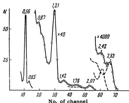
FIG. 1. Gamma-ray spectrum of  $\text{As}^{76}$ . Energies are given in Mev. Statistical errors for energies under 2.2 Mev are smaller than the size of the circles. Resolution of the hard part of the spectrum is represented by dashed curves. The ordinates are counting rates in arbitrary units.
