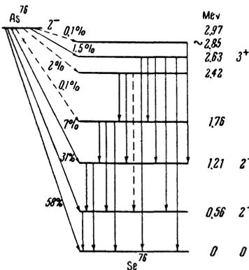
FIG. 3. Decay scheme of  $\text{As}^{76}$ .
