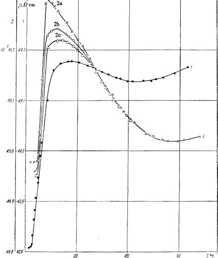
of copper-nickel alloys on temperature. Curve 1 – alloy with 58% copper; H = 0; 2a - 59.25% Cu, H = 0; 2b - 59.25% Cu, H = 1540 oe; 2c - 59.25% Cu, H = 2310 oe.
