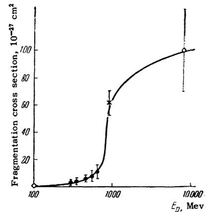
Figure 2 shows the dependence of the cross section for the production of fragments of  $Z \geq 4$  in the disintegration of Ag and Br nuclei on the energy of the incident protons, plotted from data available at the present time. The sharp increase in the cross section at energies near 1 Bev is clearly pronounced.
