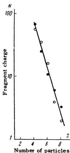
FIG. 3. Distribution of fragments by charge. ● — energy of incident protons 6.2 Bev,<sup>7</sup> ○ — energy of incident protons 9 Bev.
