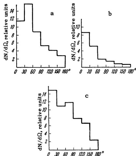
FIG. 4. Angular distribution of fragments with  $Z \geq 4$  relative to the direction of incident protons: a — disintegrations with one fragment; b — disintegrations with fast fragments, c — disintegrations with two and more fragments.
