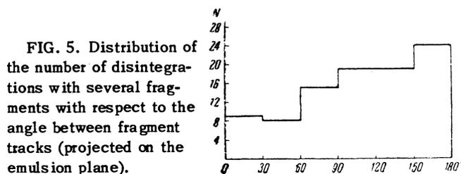
FIG. 5. Distribution of the number of disintegrations with several fragments with respect to the angle between fragment tracks (projected on the emulsion plane).
