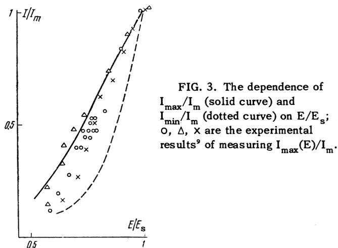
FIG. 3. The dependence of  $I_{\max}/I_m$  (solid curve) and  $I_{\min}/I_m$  (dotted curve) on  $E/E_s$ ; O,  $\Delta$ , X are the experimental results<sup>9</sup> of measuring  $I_{\max}(E)/I_m$ .
