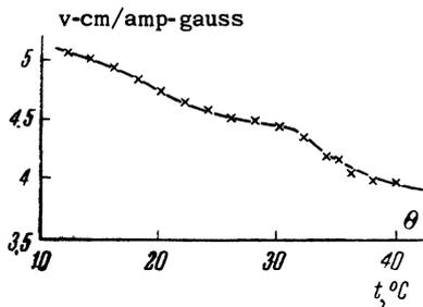
FIG. 4. Temperature dependence of the spontaneous Hall constant (10<sup>7</sup> · R<sub>s</sub>) for the nickel-zinc ferrite.
