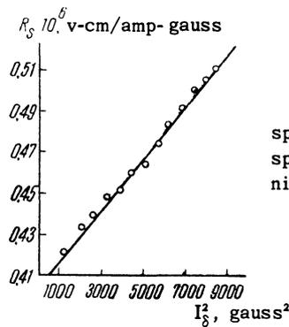
FIG. 5. Dependence of the spontaneous Hall constant on the spontaneous magnetization for nickel-zinc ferrite.
