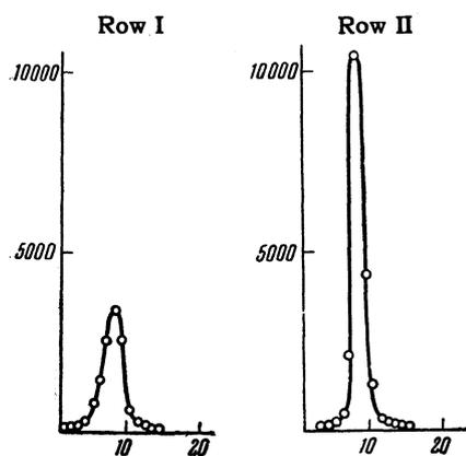
FIG. 2. Example of an event in which a newborn shower impinges on the array. Abscissa - chamber numbers; ordinate - ionization in each chamber, expressed in terms of the number of recorded particles.
