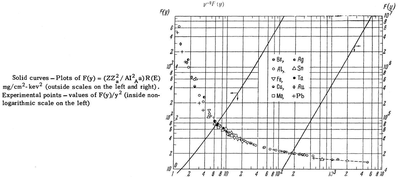
Solid curves - Plots of  $F(y) = (ZZ_a^2 / AI_A^2 a) R(E)$  mg/cm<sup>2</sup>-kev<sup>2</sup> (outside scales on the left and right). Experimental points - values of  $F(y)/y^2$  (inside non-logarithmic scale on the left)
